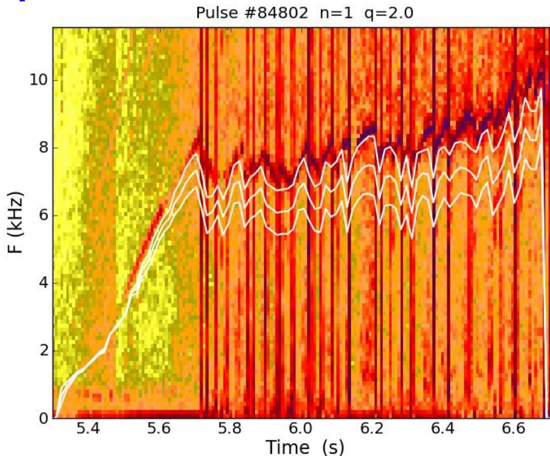
Signal from a magnetic coil inside JET
