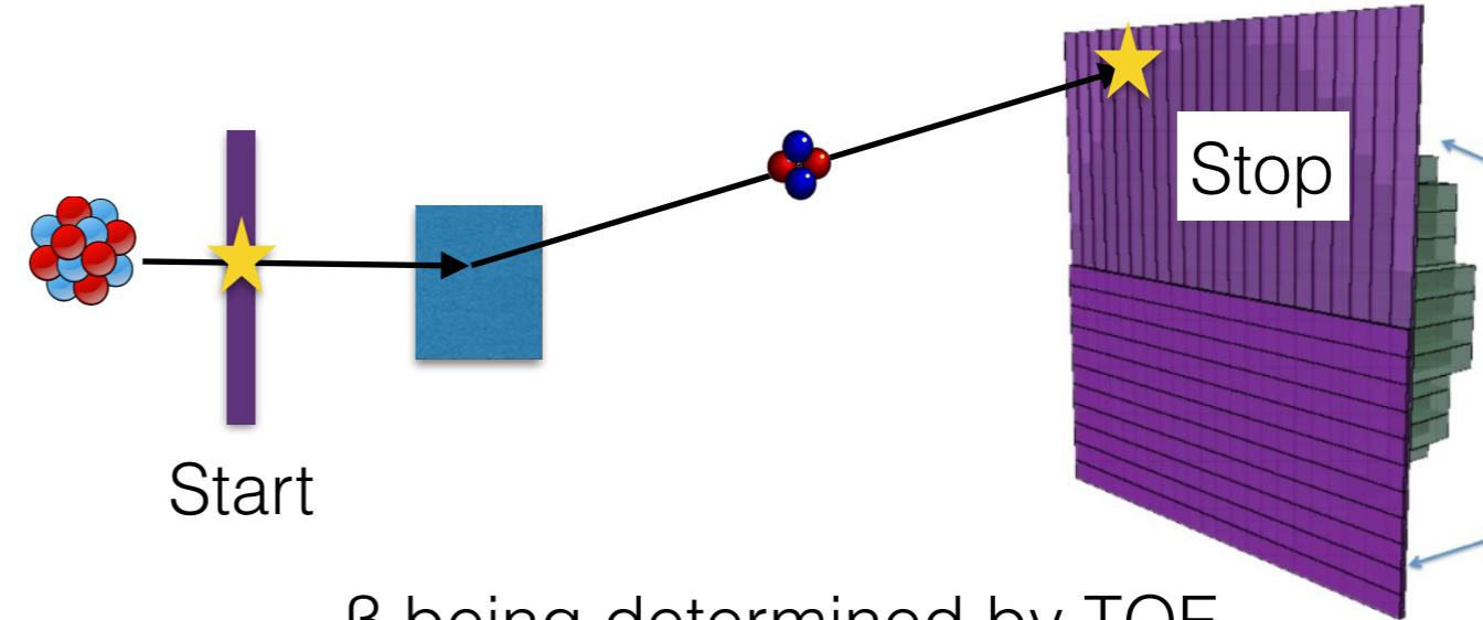
$$-\frac{dE}{dx} = \frac{\rho \cdot Z}{A} \frac{4\pi N_A m_e c^2}{M_U} \left( \frac{e^2}{4\pi\epsilon_0 m_e c^2} \right)^2 \frac{z^2}{\beta^2} \left[ \ln \left( \frac{2m_e c^2 \beta^2}{I \cdot (1 - \beta^2)} \right) - \beta^2 \right]$$
