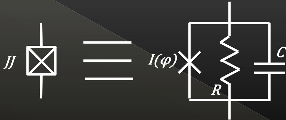
$$m_P \ddot{\phi} = -\eta \dot{\phi} - \left( \frac{I_C \hbar}{2e} \right) \sin \phi + I \frac{\hbar}{2e}$$
