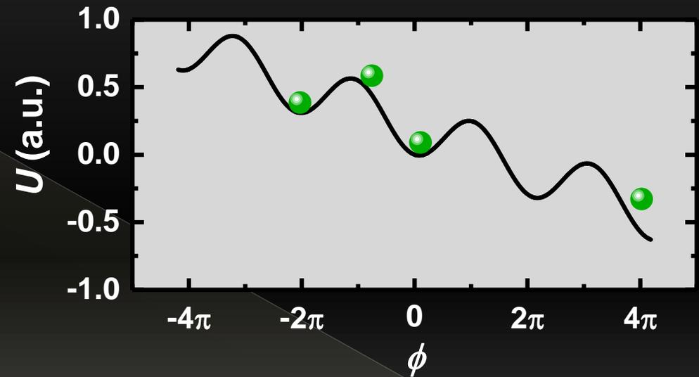
**Critical current: the minimum current that has a 100% probability of switching the superconductor to its normal state.**
