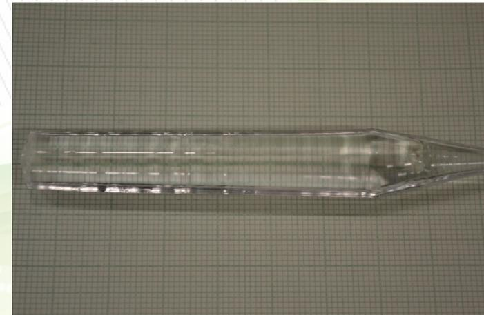
Figure 7. a typical crystal growth process using CZ method. The crystal shown in the picture is  $\text{Yb}^{3+}$  doped  $\text{LiYF}_4$ .
