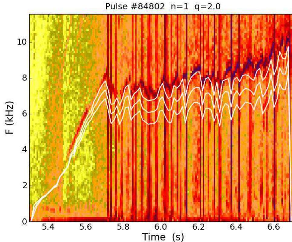
Signal from a magnetic coil inside JET
