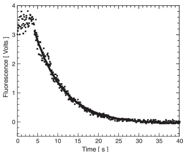
**Figure 6.** Decay of the MOT (■) as a function of time. The data are obtained by expanding the laser beam about eight times. The solid curve is an exponential fit to the data giving a lifetime of 7 s.
