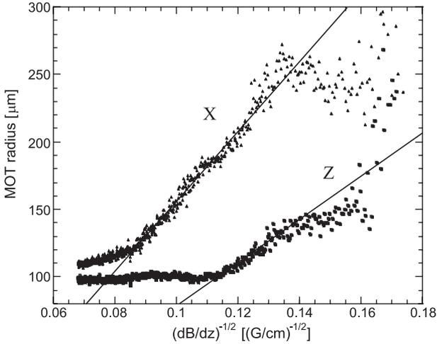
**Figure 3.** The  $x$  ( $\blacktriangle$ ) and  $z$  ( $\blacksquare$ ) MOT radii as functions of the inverse square root of the magnetic field gradient for  $\delta = -55$  MHz and total saturation parameter  $S_0 = 6$ . The straight lines correspond to a non-interacting classical gas obeying the equipartition theorem.
