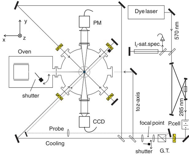
**Figure 1.** Schematic top view of the experimental set-up. In the MOT chamber atoms are captured directly from the thermal beam produced in the oven chamber. For MOT diagnostics we use a CCD camera and a photomultiplier. The  $z$ -axis indicated on the figure corresponds to the symmetry axis of the two magnet coils.
