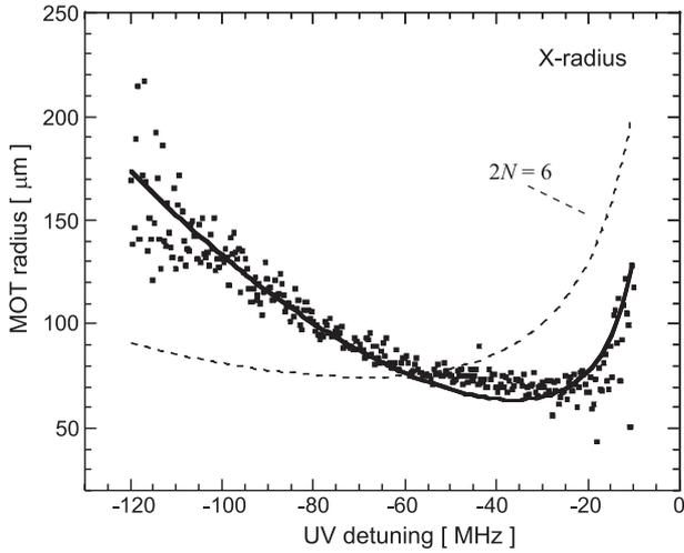
**Figure 4.** MOT  $x$ -radius (■) as function laser detuning for  $S_0 = 6$  and  $(\partial B/\partial x) = 80 \text{ G cm}^{-1}$ . The solid curve is a fit to based on equation (2) for a two-level atom. The effective saturation coefficient  $2N_0 = 0.6$  and a scaling  $c = 2.1$  on the radius. For comparison we show a fit, dashed curve, where  $2N$  is fixed to 6 and  $c = 1$ .
