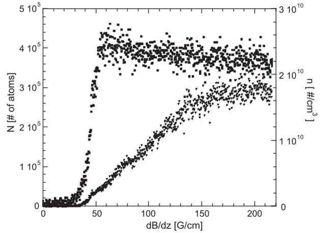
**Figure 2.** Number of captured atoms  $N$  (■) and mean atom density  $n$  (▼) as a function of magnetic field gradient in the  $z$ -direction. The laser detuning is  $\delta = -55 \text{ MHz}$  and the total saturation parameter  $S_0 = 6$ .
