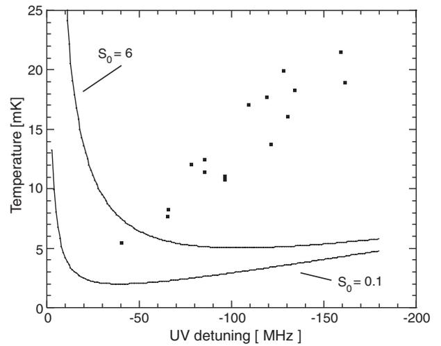
**Figure 5.** The MOT temperature (■) measured as a function of laser detuning, with  $S_0 = 6$  and  $(\partial B/\partial z) = 160 \text{ G cm}^{-1}$ . The solid curves are the prediction of Doppler theory with saturation parameters of  $S_0 = 0.1$  and 6.
